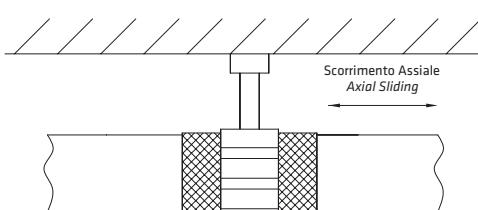
**Sliding points:** they have the function to allow the axial sliding of the pipe in both directions. They are located on a free area of the pipe surface, away from pipe fitting junctions. The collar that has the function to favor sliding should be free from parts that could cause cuts. The sliding points, arranged according to appropriate numbers and distances, ensure the maintenance of the rectilinear geometry of the installation under thermal stress.
