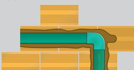
TORO 25 can be installed directly into concrete walls, plaster and lime. The comprehensive strain and stress arising from a temperature dependant linear expansion is not critical as they are absorbed through the material.
