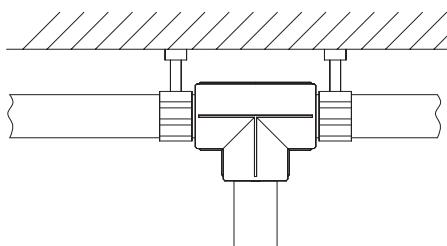
**Fixed Points:** they have the function to prevent pipes from sliding and to create a rigid connection between pipes and walls. They are made up of rigid collars endowed with an inside rubbery coating (or similar), aimed at avoiding any cut. The fixed points are placed next to direction changes (branches, elbows, etc.), in order to avoid a stress concentration in those areas.
